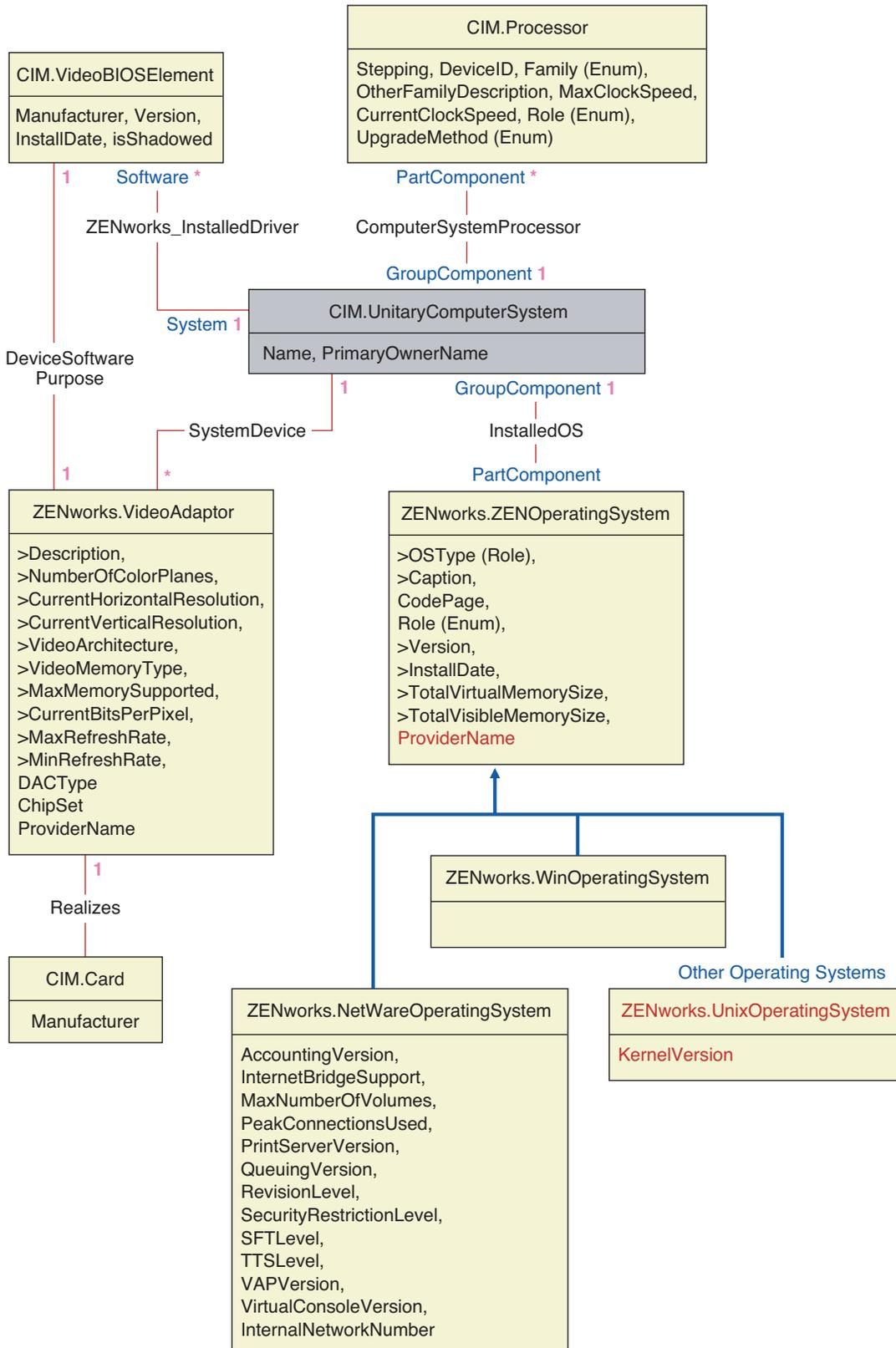
Figure 15-1 shows how the CIM schema maps to a relational DBMS schema. The classes are shown with the class name as the box heading. The associations are labeled within the lines between two classes.
