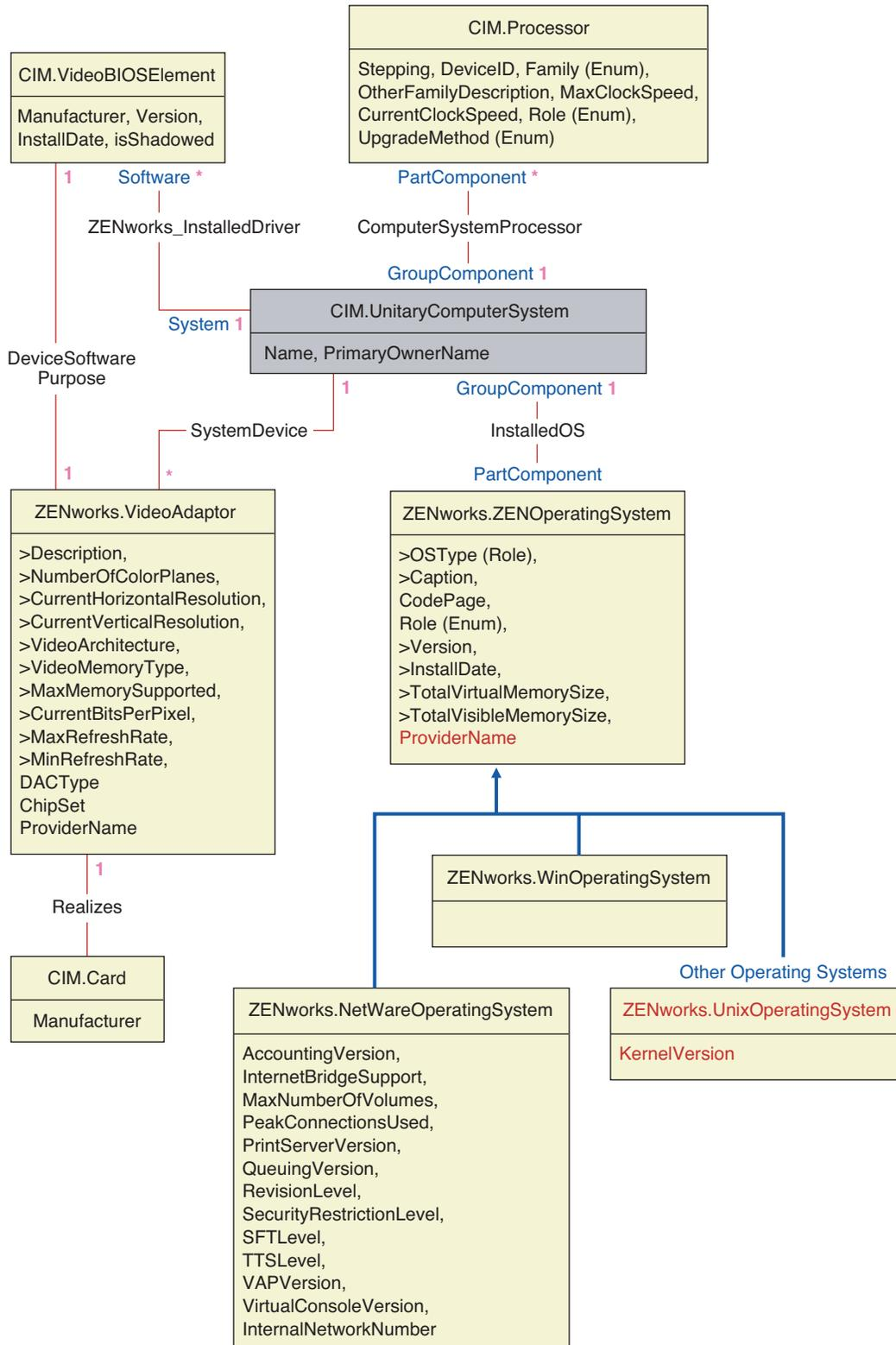
**Figure 15-6** Schema for Inventory Scanner and NetWare Client
