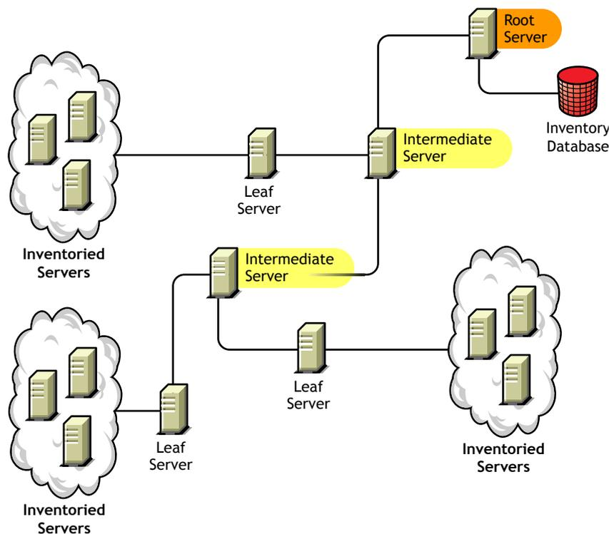
In this illustration, there are many Leaf Servers and Intermediate Servers at different levels. The Intermediate Server is a staging server for uploading the scan information to the next-level server. The last Intermediate Server is attached to the topmost Root Server. This scenario is typical if there are many Leaf Servers in different geographical locations. All the Leaf Servers move the inventory information to the Intermediate Server.
