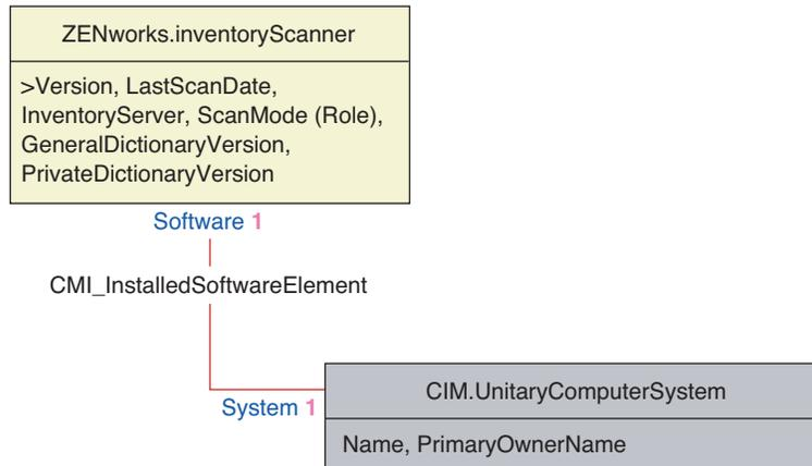
**Figure 15-7** Schema for Chassis and System Information
