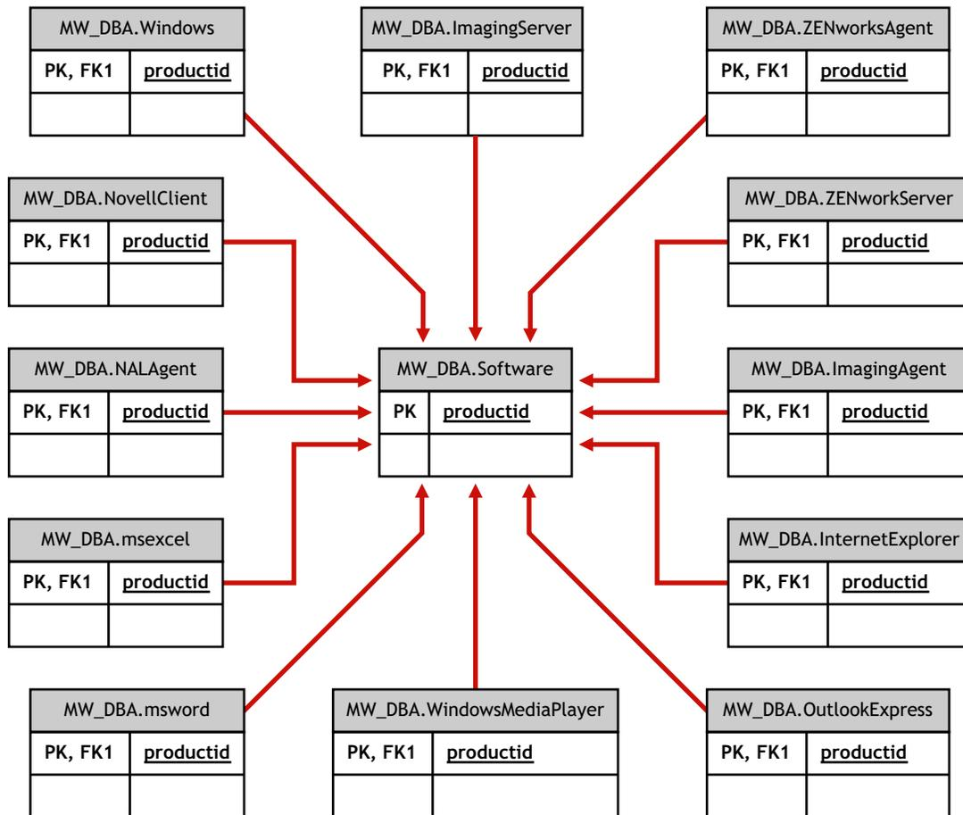
**Figure 15-19** Schema for Software Sub-classes
