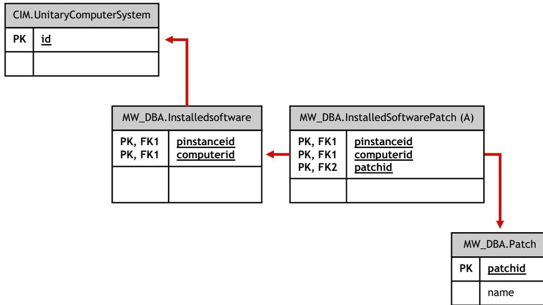
In [Figure 15-15](#), class MW\_DBA.Patch associates to MW\_DBA.InstalledSoftware using the association MW\_DBA.InstalledSoftwarePatch with MW\_DBA.InstalledSoftwarePatch.pinstanceID pointing to MW\_DBA.InstalledSoftware and MW\_DBA.InstalledSoftwarePatch.PatchID pointing to MW\_DBA.Patch. The relationship between the two classes is one to many. This means a software might have zero or more patch information.
