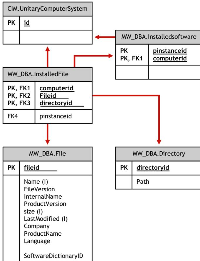
In **Figure 15-16**, class `MW_DBA.File` associates to `MW_DBA.InstalledSoftware` using the association `MW_DBA.InstalledFile` with `MW_DBA.InstalledFile.pinstanceID` pointing to `MW_DBA.InstalledSoftware` and `MW_DBA.InstalledFile.fileID` pointing to `MW_DBA.File`. The relationship between the two classes is one to many. This means a software might have zero or more file information.
