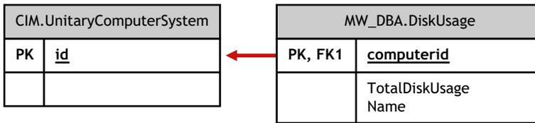
In the above illustration, MW\_DBA.DiskUsage has the computerID column foreign key references to the CIM.UnitaryComputerSystem.ID. The MW\_DBA.DiskUsage table contains the total disk usage and the file extension name.
