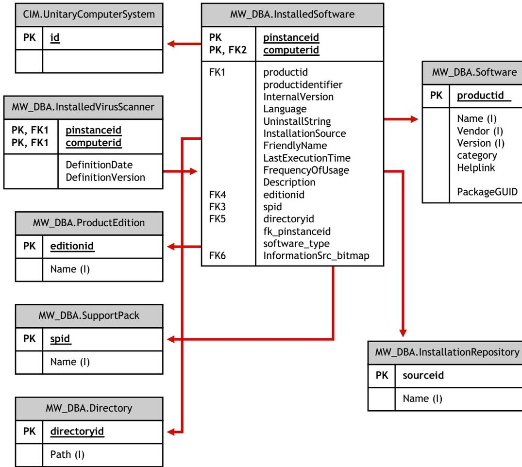
In **Figure 15-14**, class MW\_DBA.Software associates to CIM.UnitaryComputerSystem using the association MW\_DBA.InstalledSoftware with MW\_DBA.InstalledSoftware.ComputerSystem pointing to CIM.UnitaryComputerSystem and MW\_DBA.InstalledSoftware.ProductID pointing to MW\_DBA.Software. The relationship between the two classes is one to many. This means a computer system might have more than one software information.
