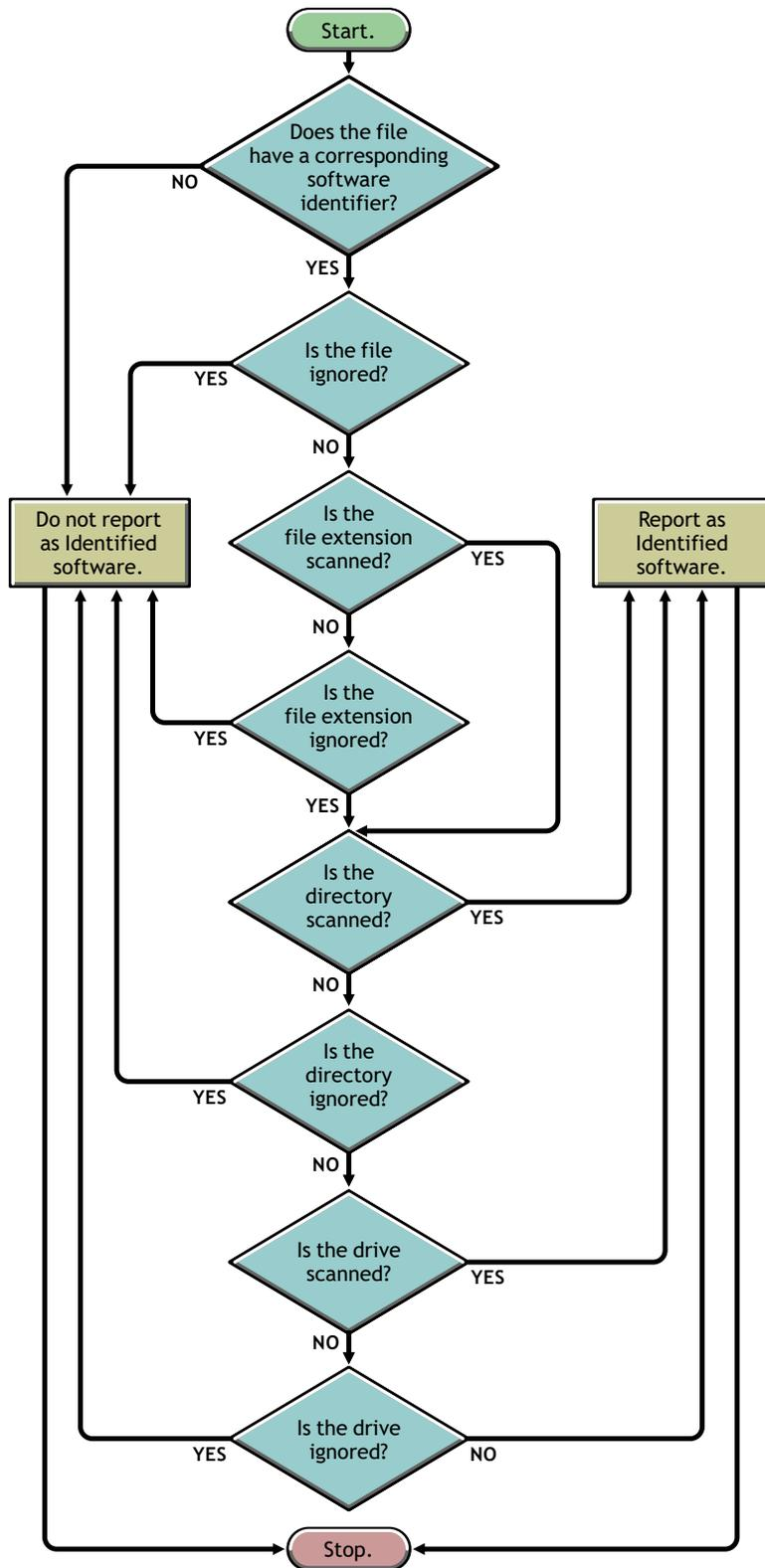
**Figure 16-2** Precedence of Software Dictionary rules in the Software Scanning category
