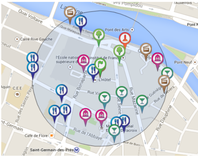
Figure 6. The Pop Radius is centered on the POI that has been clicked on. All the POIs inside this area are shown with an icon according to their category (or type of attraction). The starting point has a green flag. By double clicking on a POI, it adds it to the POI list and makes it the temporary ending point.
