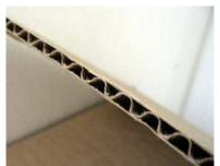
Corrugated cardboard is a good example of how a truss design makes the overall structure stronger.
