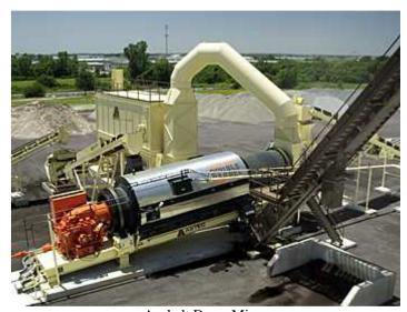
Asphalt Drum Mixer Source: http://obr.gcnpublishing.com/articles/mar06e.htm
