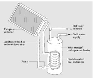
"An indirect solar hot water system." U.S. Department of Energy www.eere.energy.gov/de/solar\_hotwater.html
