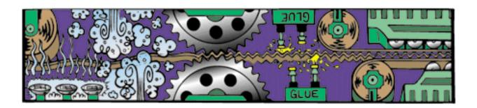
The **web**, or long sheet of paper unwinding from the roll, is drawn between a pair of gear-like cylinders called **corrugating rolls**. This shapes the paper into a series of precise waves. Glue is applied to the tips of these flutes on one side — just the right amount, and at just the right places — and the flute tips are pressed against a flat liner.
